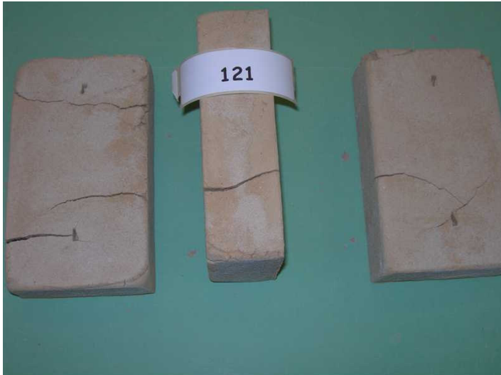
Figure 3: Crack formation in products made with the addition of 0.4 % KP 1131
